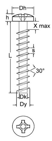
Part No. example: 0693x10-PH - 3mm diameter x 10mm long
