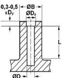
The table above shows the recommended hole dimensions. The first few parts should be tested under controlled conditions to assess the effects of: Local surface finish, fillers, mould flow, meld and welds lines.
