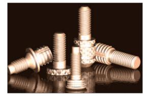
A range of Tappex inserts with male threads or studs is available based on the same body design and installation features of the female equivalent. Thus the basic forms of Trisert, Multisert or HiMould, can be produced in Unheaded and Headed versions with the same Short, Regular and Long body lengths as the relevant female insert, with a defined stud length.
