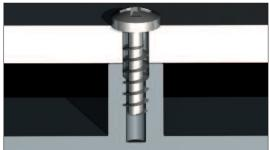
The Tappex TPX thread forming screws (not thread cutting) are designed to be used in most thermoplastic materials. These screws can be installed into drilled or moulded holes in a wide variety of applications.
