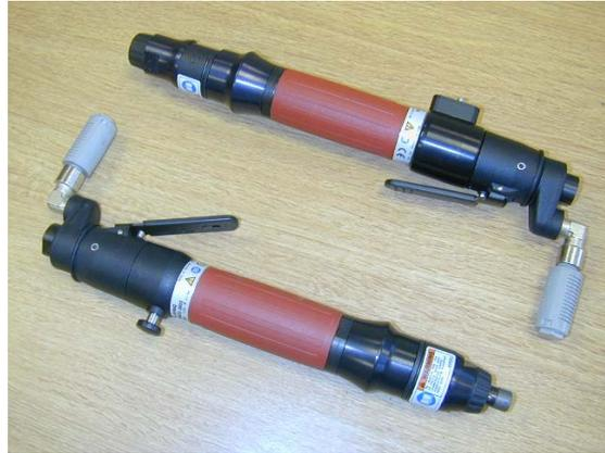
The Tappex FlexiArm installation machine consists of a pantograph arm with a Desoutter pneumatic screwdriver attached. The screwdriver can be 510rpm automatic reverse, 1100rpm automatic reverse, or a 510rpm manual reverse depending upon the size of the insert and the material it's being installed into.
