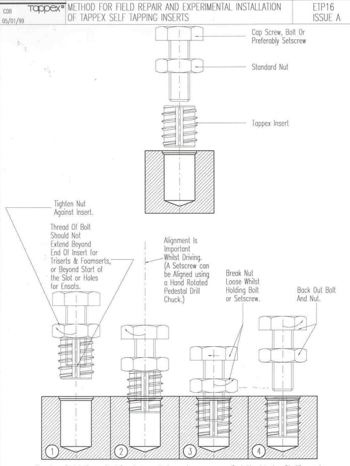
The above installation method is only suggested as a temporary expedient. Hand tools, with Alignment Bushes, are available for low volume applications, Production Drivers for medium to high volumes.
